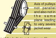
Note: The belts should be properly tensioned as specified in IS 2494 & BS 1440 for the various sections of the belts to get optimum life Maintenance of V - Belts
